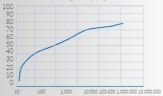
The pore structure of CCC GAC AQUA SORB 8x30 carbon is illustrated below, where cumulative pore volume is plotted against pore diameter. Correlation studies have shown that adsorption capacity is determined in part by total pore volume and pore size distribution. Color bodies and high molecular weight organic impurities require pores within the 20 to 500 Angstrom Unit range, while odors and low molecular weight impurities require pores smaller than 20 Angstrom Units.
