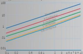
The pressure drop per foot of bed depth for CCC GAC AQUA SORB 8X30 carbon for varying flow rates at different viscosity levels is illustrated. This data was obtained in down-flow column operation with a normal packing arrangement in which the carbon was pre-soaked in hot liquid and charged to the column as a slurry. The bulk density of the charged carbon was calculated to be approximately 30 lb/ft3.
